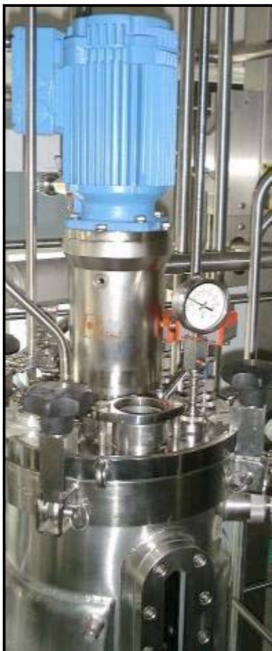
bio-M AMR 550 with a 40 L Cellculture bioreaktor
